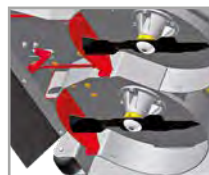
Mulching cut Closed cutting chamber
