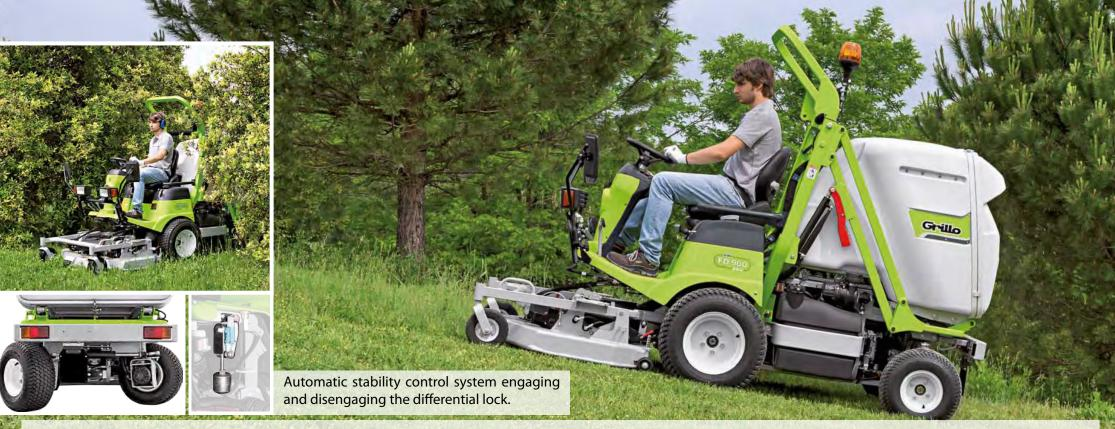
The innovative permanent 4WD ensures, via the hydraulic differential, **maximum grip under all working conditions and even on tight turns without damaging the grass.** Perfect weight distribution combined with the automatic and/or manual differential lock make this mower safe and steady when cutting on slopes. The rear axle tilts allowing 4WD on uneven ground as well.
