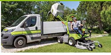
The hydraulic services of both the grass-catcher and cutting deck are activated via practical levers fitted with safety system devices and are located on the dashboard. It is very easy and quick to empty grass into a truck and also easy to raise the cutting deck when negotiating obstacles or kerbs.
