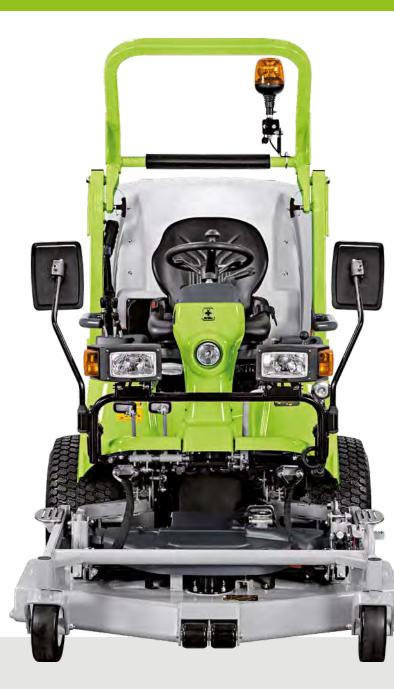
The FD 900 is equipped with a Yanmar 3TNV80F diesel engine, 25 HP, three cylinders, compliant with the directives EC (NRMN) STAGE V (EUROPE) and EPA FINAL TIER 4 (USA), mounted on shock-absorbers into a very robust frame, designed to protect the machine main components.
