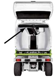
Easy rear access to the hydraulic components such as the service pump and the drain-block. The grass grid can be removed for cleaning.
