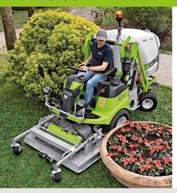
The FD 13.09 is a compact mower with a very narrow wheelbase, equipped with power steering and a turning radius of only 31 cm.
