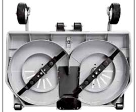
Mulching kit as a standard feature on cutting decks with collection
