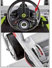
Hydraulic and continuous cutting height adjustment
